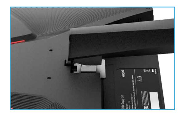
Push the monitor stand to install it, and make sure the hook is "clicked" to confirm it is in place.
